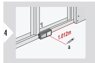
Start measuring. Move device slowly along the stake out line. The distance to the previous/next stake out point is displayed.
