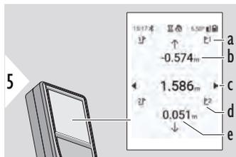
When approaching a stake out point to less than 18 mm the value of the stake out point is frozen and arrows appear on the side of the display for marking purposes.
