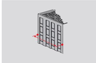
The result is shown in the main line. Pressing the measuring key for 2 seconds in the function activates automatically minimum/maximum measurement. We recommend using the Pythagoras only for indirect horizontal measuring. For height measuring (vertical), it is more precise to use a function with inclination measurement.
